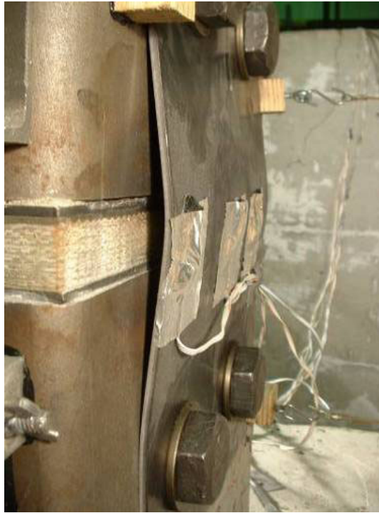
Figure 126. Photographs of Column 5 – Cycle 18b west fuse plate buckling.
