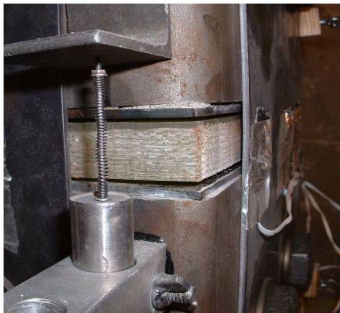
b.) West joint opening during pull half-cycle
