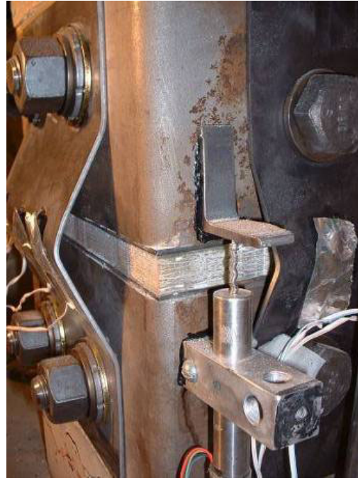
b.) East fuse plate buckling
