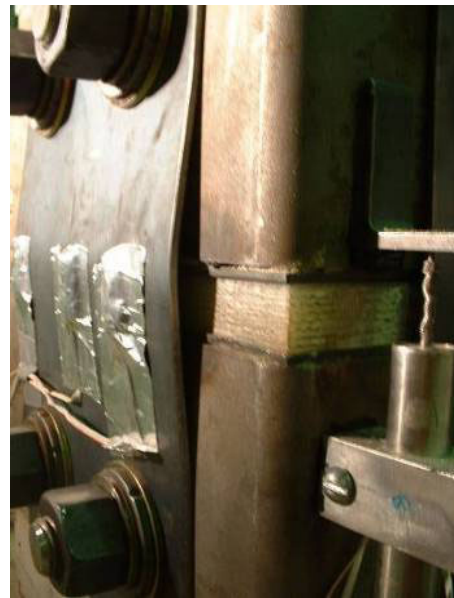
b.) East fuse plate buckling
