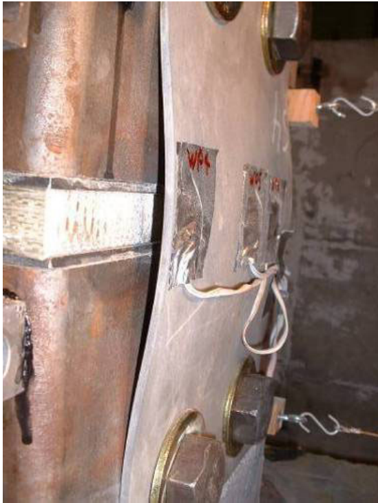
a.) West fuse plate buckling
