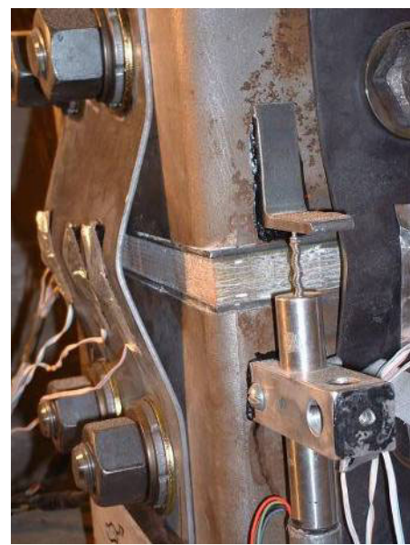
d.) Northeast corner fuse plate buckling
