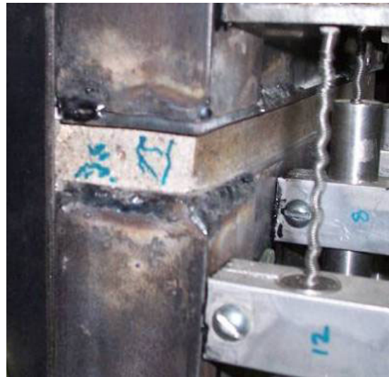
b.) Northeast corner bearing plate compression damage
