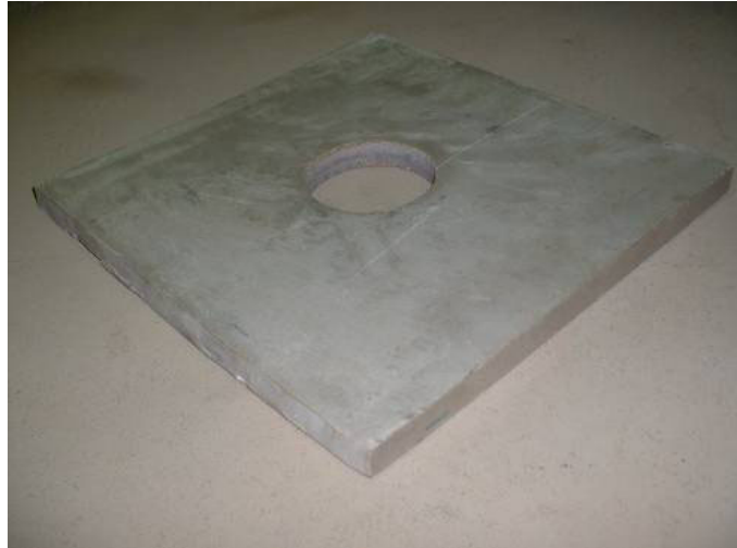
Figure 63. Photograph of epoxy grout plate.
