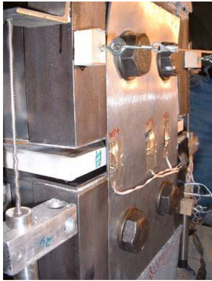
a.) Northeast corner joint opening
