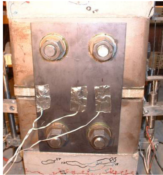
b.) East joint opening during push half-cycle
