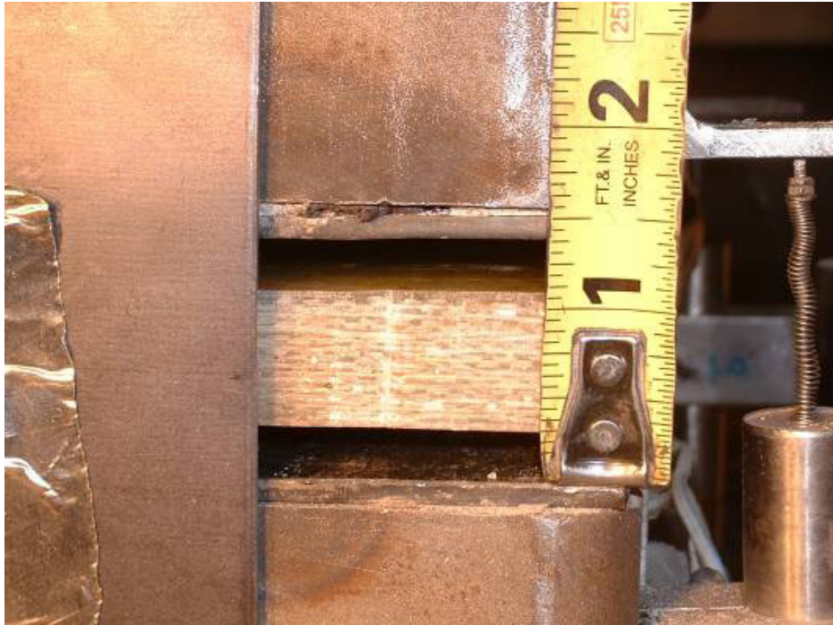
a.) East joint opening during push half-cycle
