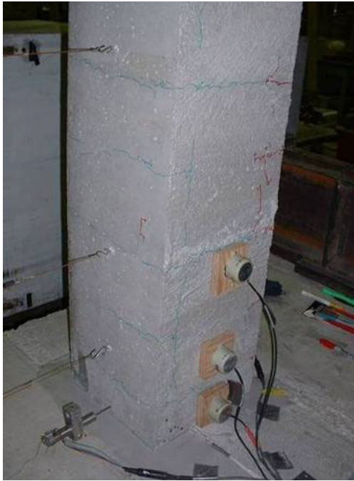
a.) Southwest corner view of progressive cracking
