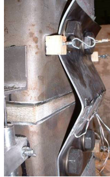
b.) West fuse plate buckling
