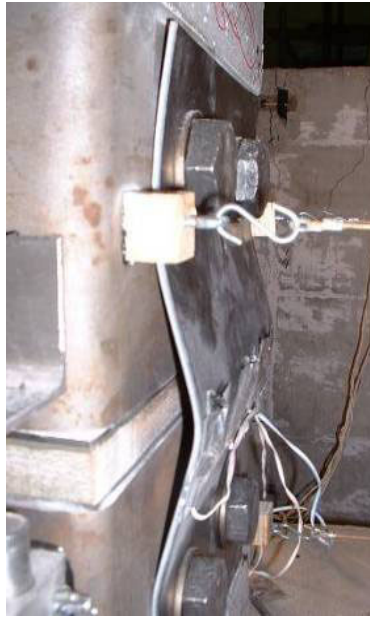
a.) West fuse plate buckling
