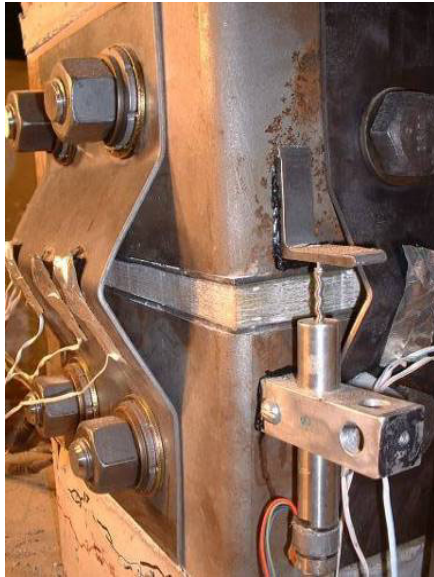
a.) East fuse plate buckling
