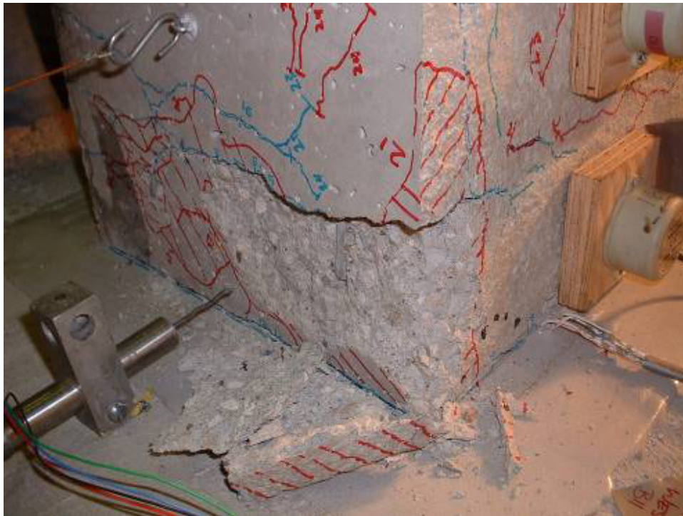
Figure 78. Photograph of Column 1 – Cycle 24 damage to southwest corner
