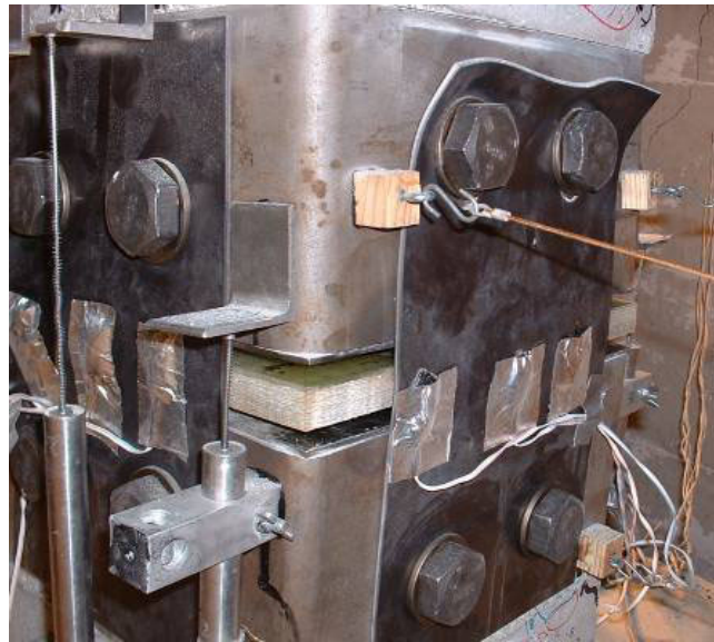
b.) West joint opening and bearing of west fuse plate on bolts
