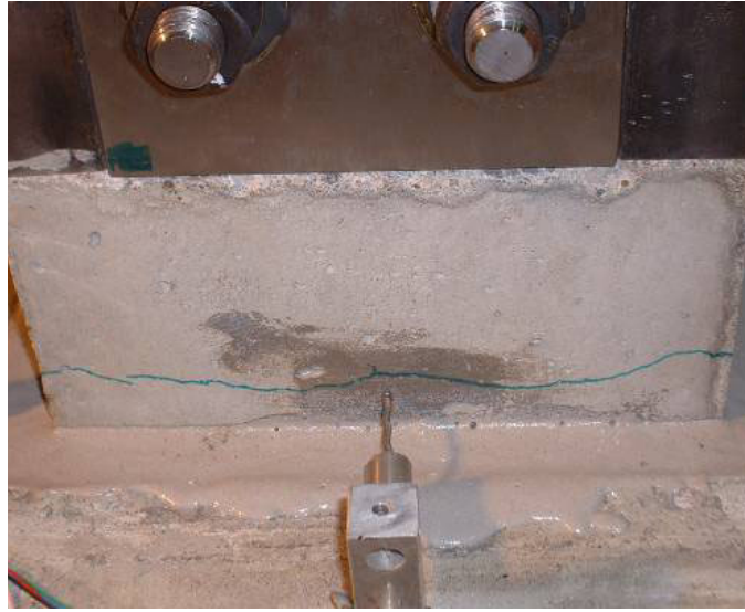
b.) East base initial cracking
