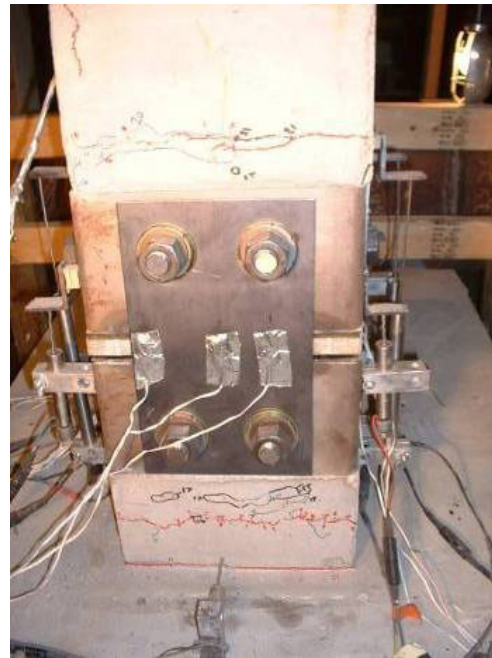
d.) East joint opening and segment damage
