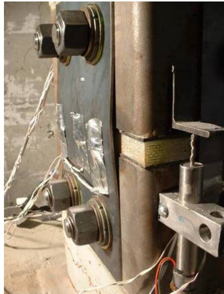
b.) East plate initial buckling
