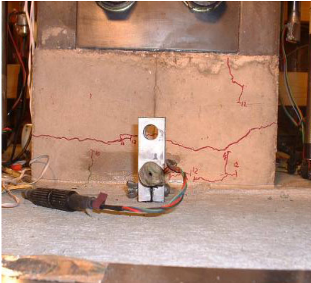
a.) East base cracking
