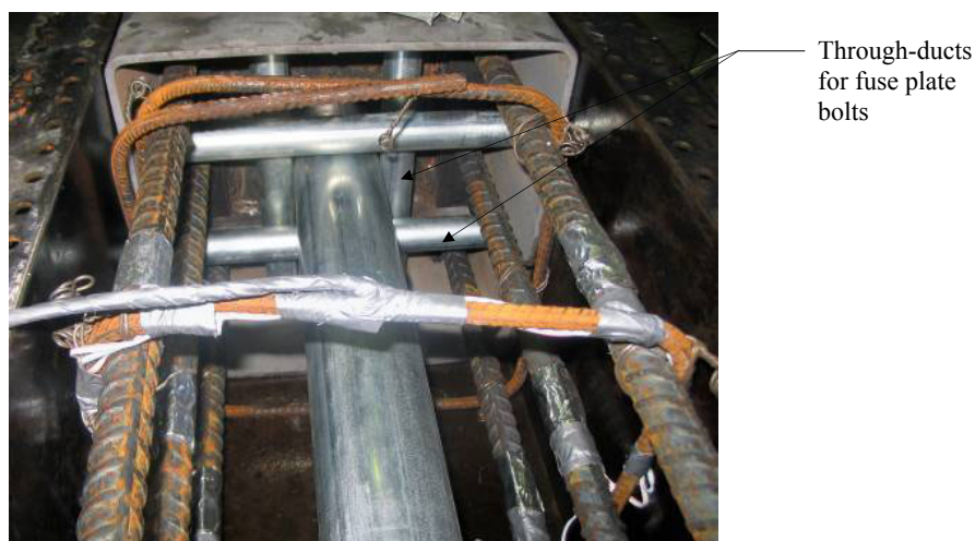
Figure 55. Photograph of Column 5, 12 ft. segment collared end.
