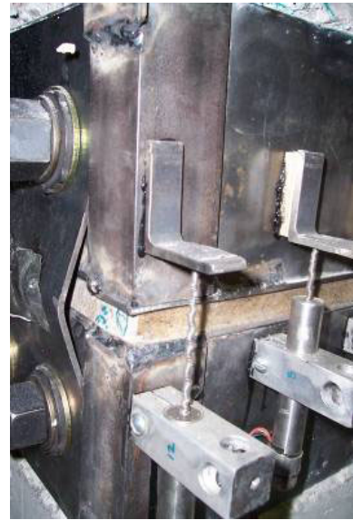
d.) Northeast corner fuse plate buckling
