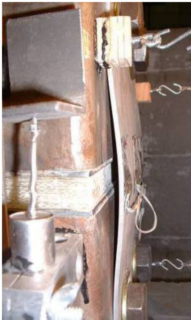
a.) West fuse plate buckling
