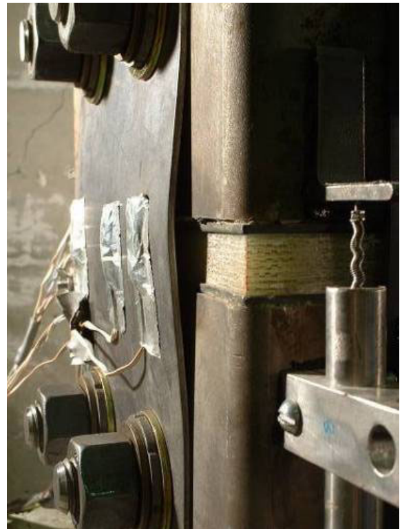
b.) East plate buckling in compression
