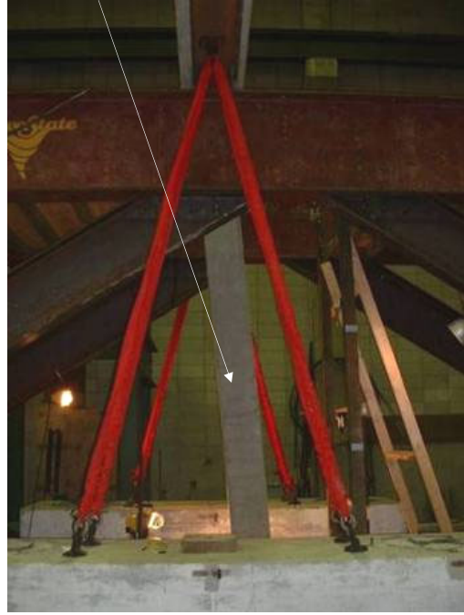
b.) Column deformation on pull half-cycle
