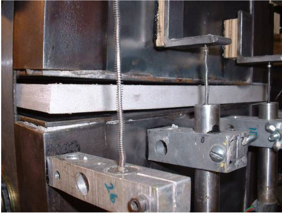
Figure 102. Photograph of Column 3 – Cycle 21b joint opening during push half-cycle.
