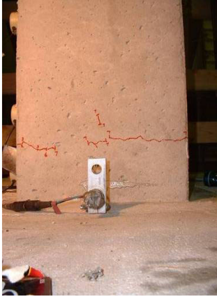
a.) East face initial cracking
